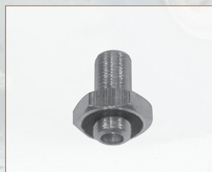
VLH-EX-AD1 Adaptor to convert large bore to standard bore. Fits .302-32 thread
